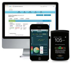
Embedded cellular solutions, which consist of a blood glucose meter capable of transmitting clinical values and receiving messaging from a back-end cloud server, thus completing the feedback loop between patient and caregiver.
